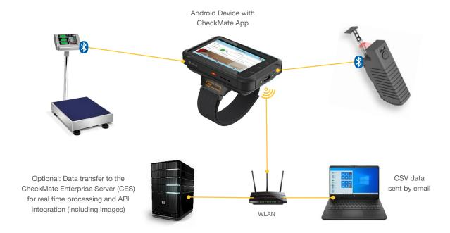
Cubetape POS for easy entry of barcoded parcel ID and parcel dimensions. Filling the fields: Barcode, L, W, H and Weight. Several scales models can be integrated.
